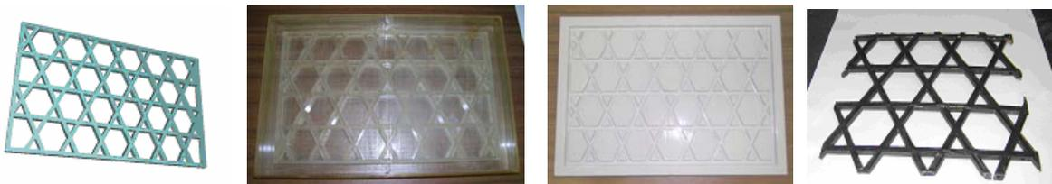
Fig. 15. Flat anisogrid element manufacturing procedure
