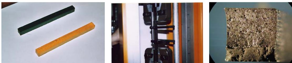
Fig. 11. Samples produced, traction test facility, optical analysis of the fracture section
