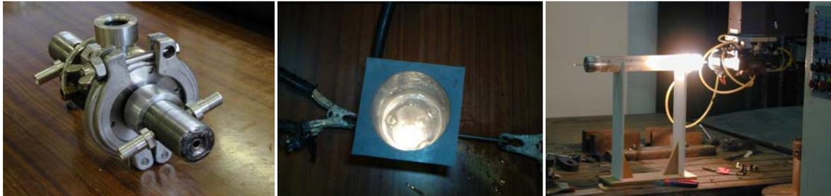
Fig. 1. The arc discharge and laser ablation facilities developed
