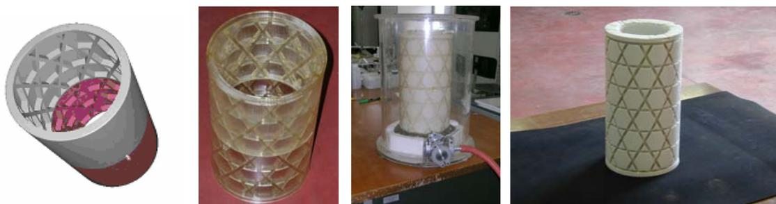
Fig. 16. Cylindrical anisogrid element manufacturing procedure
