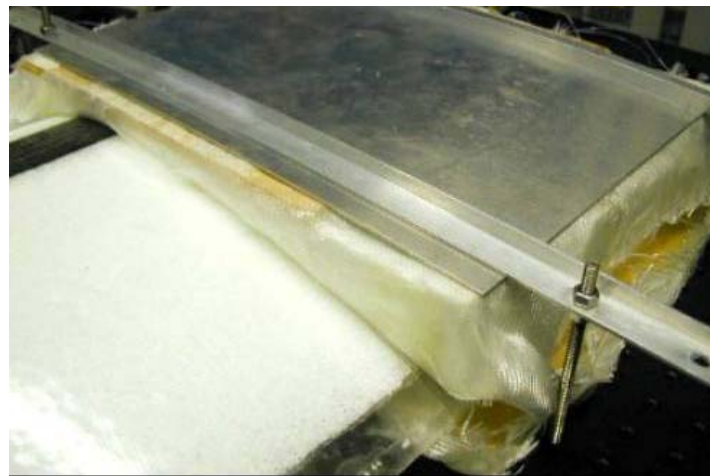
Figure 3b. Photograph of a detail of the clamped end of the wing.
