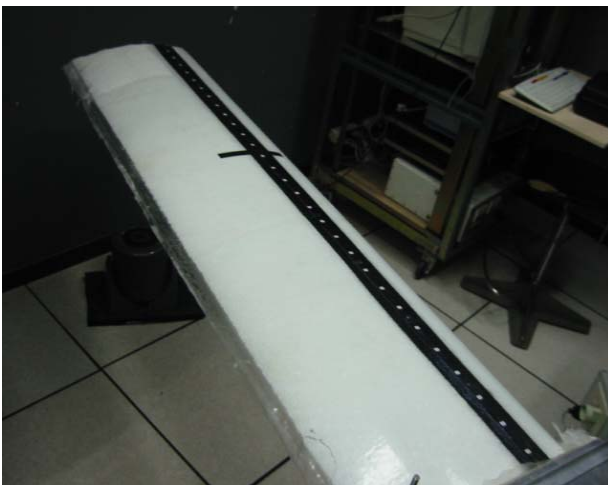
Figure 3a. Photograph of the wing. In white is the body of the wing, in black is the spar.
