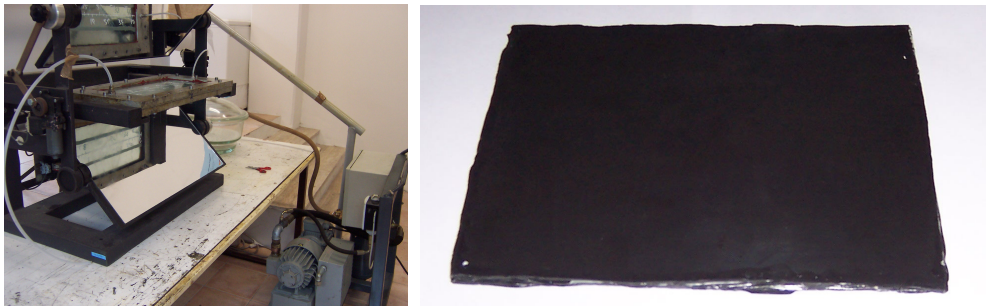
Fig. 3.4 VARTM methods developed for the manufacturing of the nanostructured polymeric composite plate
