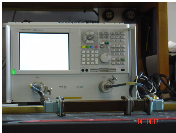
Fig. 4.1 Agilent Portable Network Analyzer (PNA) E8363B – experimental set up
