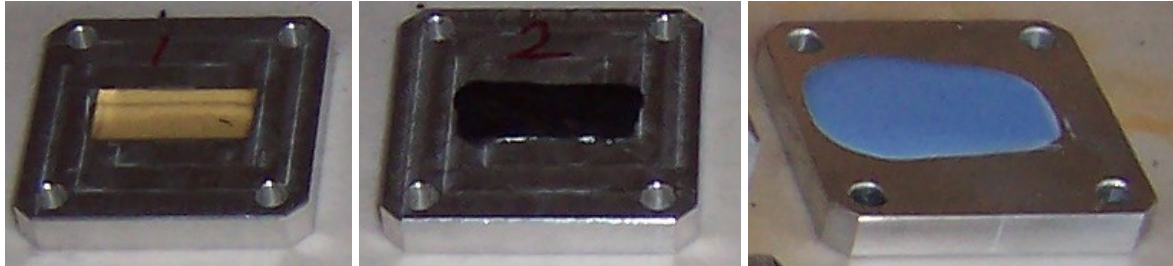
Fig. 4.2 samples: dielectric host (left), with graphite (centre) and silicone (right)
