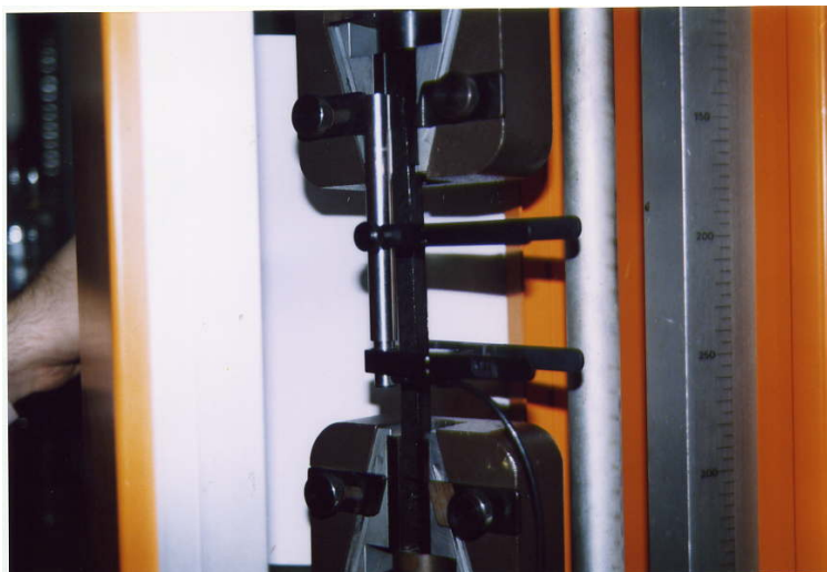
Fig. 3.2 mechanical test of the nanostructured composite samples
