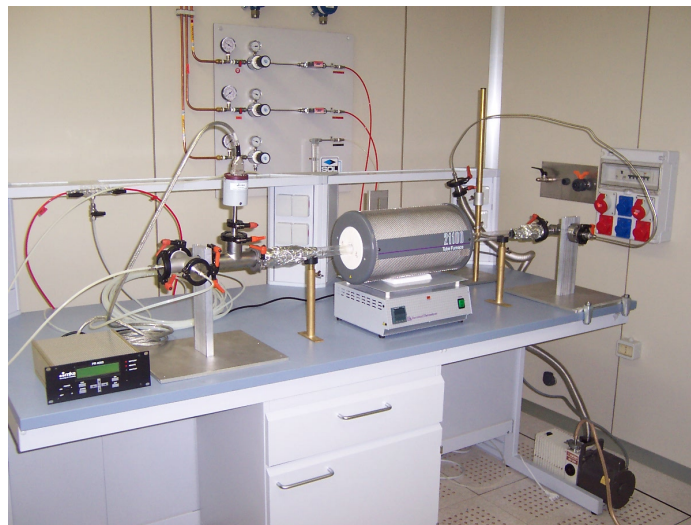
Fig. 3.12 Thermal CVD facility developed [23]
