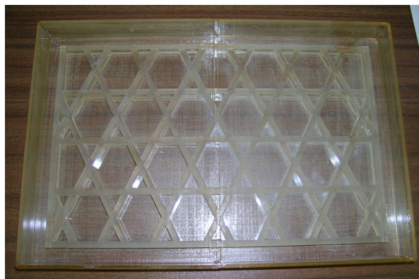
fig. 7.5 rapid prototyping positive mould
