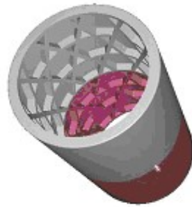
fig. 5.14 3D - CAD design of the anisogrid lattice cylindrical element and rapid prototyping positive mould
