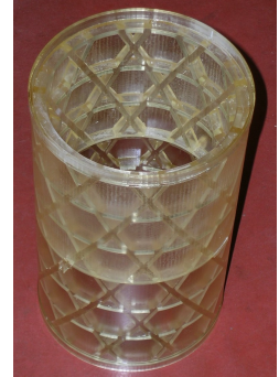
fig. 5.14 3D - CAD design of the anisogrid lattice cylindrical element and rapid prototyping positive mould
