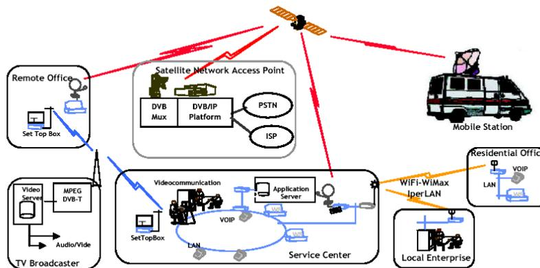
Figure 2 – Satellite and Wireless Network Architecture
