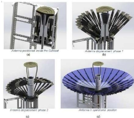
Figura 12: antenna deployable in banda Ka per ISL LEO-GEO
