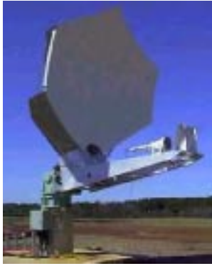
Figure 9: NCC Ka Antenna 3.8 m (courtesy of Vertex)
