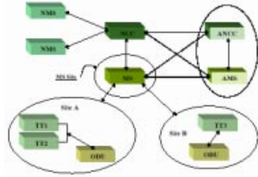
Figure 4: Redundant network configuration
